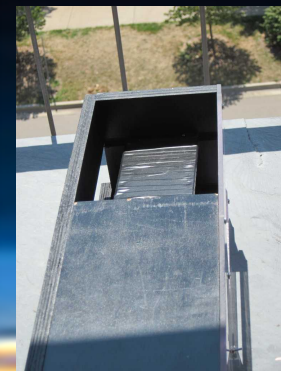
View of one of the scintillating panels wrapped in aluminum foil
