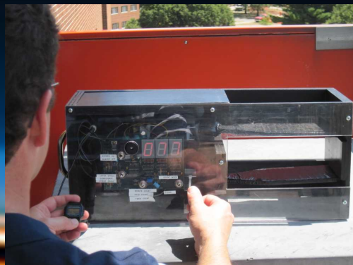
The Scintillator Counter
