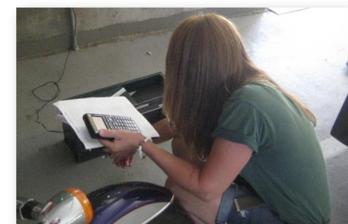
Cosmic ray detector was set for a coincidence setting. Three, three-minute trials were conducted at each location.
