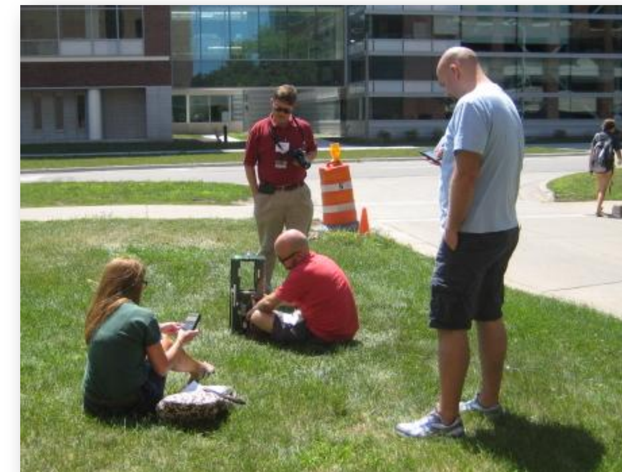
Outside of the parking garage (no shielding effects) data was collected with scintillators parallel and perpendicular to the ground to gather control data.
