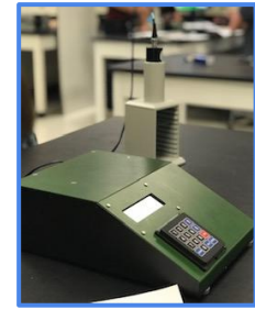
The Geiger-Muller Tube setup
