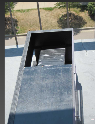
View of one of the scintillating panels wrapped in aluminum foil
