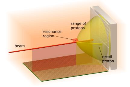
Figure 8: Configuration of ACTAR for the measurement of resonant reactions. Ancillary detectors are placed at forward angles to intercept charged particles escaping the gas volume. The range of protons is calculated from their energy after the scattering (see Fig. 7).
