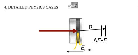
Figure 6: Resonant reactions in a thick target in inverse kinematics: the energy of the beam is degraded through the target, and reactions mainly occur at centre of mass energies corresponding to a resonance. The beam is stopped in the target, while the light recoil escapes and is detected and identified at small angles.
