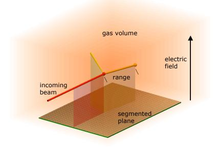
Figure 2: Arrangement of an active target detector.
