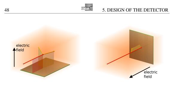
Figure 18: Left: planar configuration, with the field perpendicular to the beam direction. Right: axial configuration.
