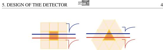
Figure 16: Effect of the pad shape: on the square pads (right) the two tracks induce the same signal. By using a triangular form (right), the two signals differ, because the fraction of the projection on the pad depends on the position. The information can be correlated with that of neighbouring pads to increase the resolution.
