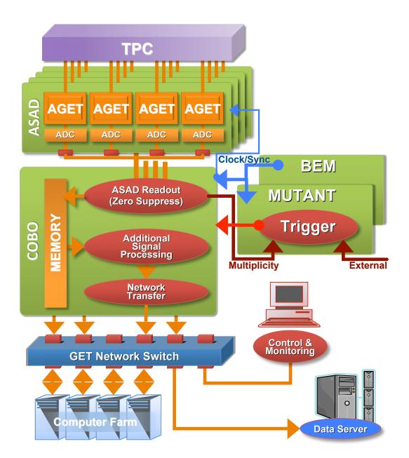
Figure 19: Schematic view of the GET system and its different parts. The ASAD and COBO modules read out and process the data, sending them over a network after validation by a multiplicity processing system.
