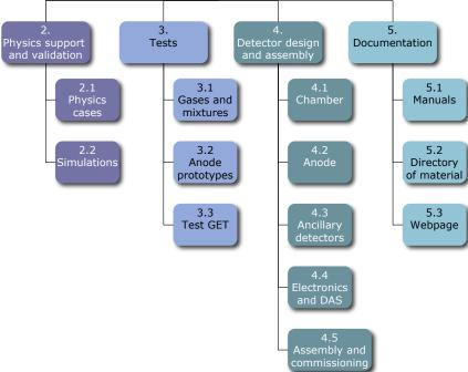
Figure 20: Work Breakdown Structure for the ACTAR project.
