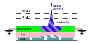
Figure 17: Scheme of a double GEM amplifier and anode with resistive layer (from [68]). The charge is distributed on the neighbouring pads.
