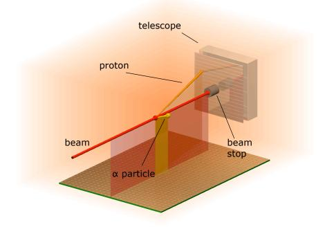
Figure 11: Configuration of ACTAR for the measurement of inelastic scattering on  $\alpha$  particles and detection of charged particles emitted in the in-flight decay of the IS-GDR. The beam can be either stopped before the telescope (as shown), or leave the gas detector through a central hole in the telescope.
