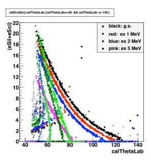
Figure 5: Particle identification for p, d, and t in the Si-CsI telescopes located outside the active gas volume: the detected energy is plotted versus their calculated scattering angle. The colour codes are the same as in Fig. 4.
