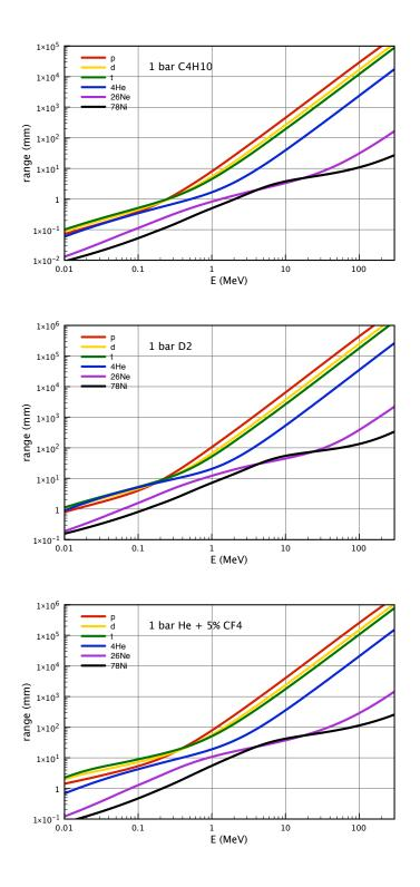
Figure 22: Range of particles in gases of interest for ACTAR.
