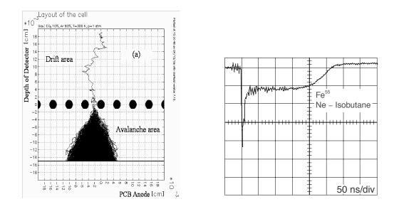
Figure 14: Left: simulation of the avalanche of an electron as it comes to the region of high field. Right: corresponding current pulse with the fast electron signal and the slower ion signal (taken from Ref. [63]).
