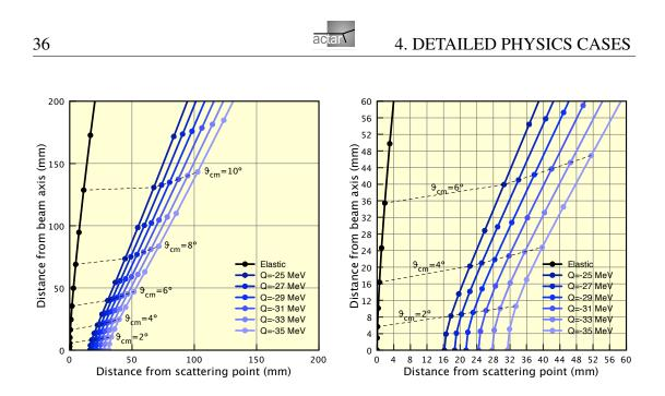
Figure 9: Loci of  $\alpha$  particles scattered (at the origin point of the plots) by <sup>56</sup>Ni at 50 MeV/nucleon, both elastically and inelastically (Q = -25 to -35 MeV), after energy loss in a He-CF<sub>4</sub>(5%) gas at 1 bar pressure. The energy loss calculations have been performed using SRIM [55]. In the blow-up on the right panel, the grid reproduces the maximum expected pad size for ACTAR.
