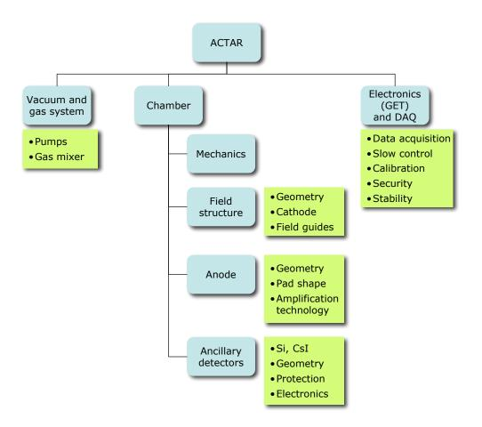
Figure 12: Product Breakdown Structure of the ACTAR detector.
