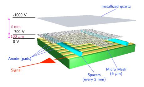
Figure 13: Arrangement of a Micromegas electron amplification device.
