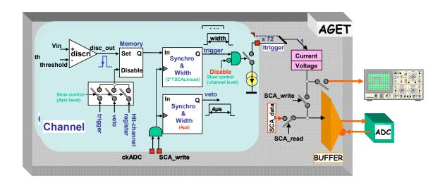
Fig 1: Schematic of the trigger signal management.
