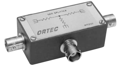
MT050 50-Ω Matched Tee Signal Splitter One input provides two equal half-amplitude outputs and still preserves 50-Ω termination; reflection, typically 10% (dc to over 500-MHz equivalent bandwidth); rise time, 1 ns; continuous input power, 1 W.
