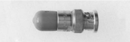
T50 Terminator, 50 Ω, BNC. Provides a high-quality 50-Ω (±1%) 1/2-W termination.
