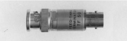
TF50 Feedthrough terminator, 50 Ω, BNC. Provides 50-Ω (±2%) 1-W feedthrough termination of 50-Ω cable at high-impedance inputs.
