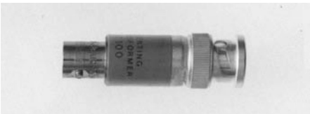
IT100 Inverting Transformer A compact pulse-inverting transformer for use in a 50-Ω system; has low distortion; good linearity, freedom from overload effects, 0.8-ns rise time capability, and 7% tilt in 100 ns.
