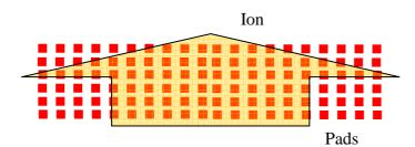
First case: Ion event is stored then sent to DAQ before 2p radioactivity Readout time:  $512x \text{ [n channel + 3]}x\text{Trck} + 79x\text{Trck} = 64.6 \,\mu\text{s} + 20.48 \,\mu\text{sxnchannel}$ [Trck = 40 ns]
