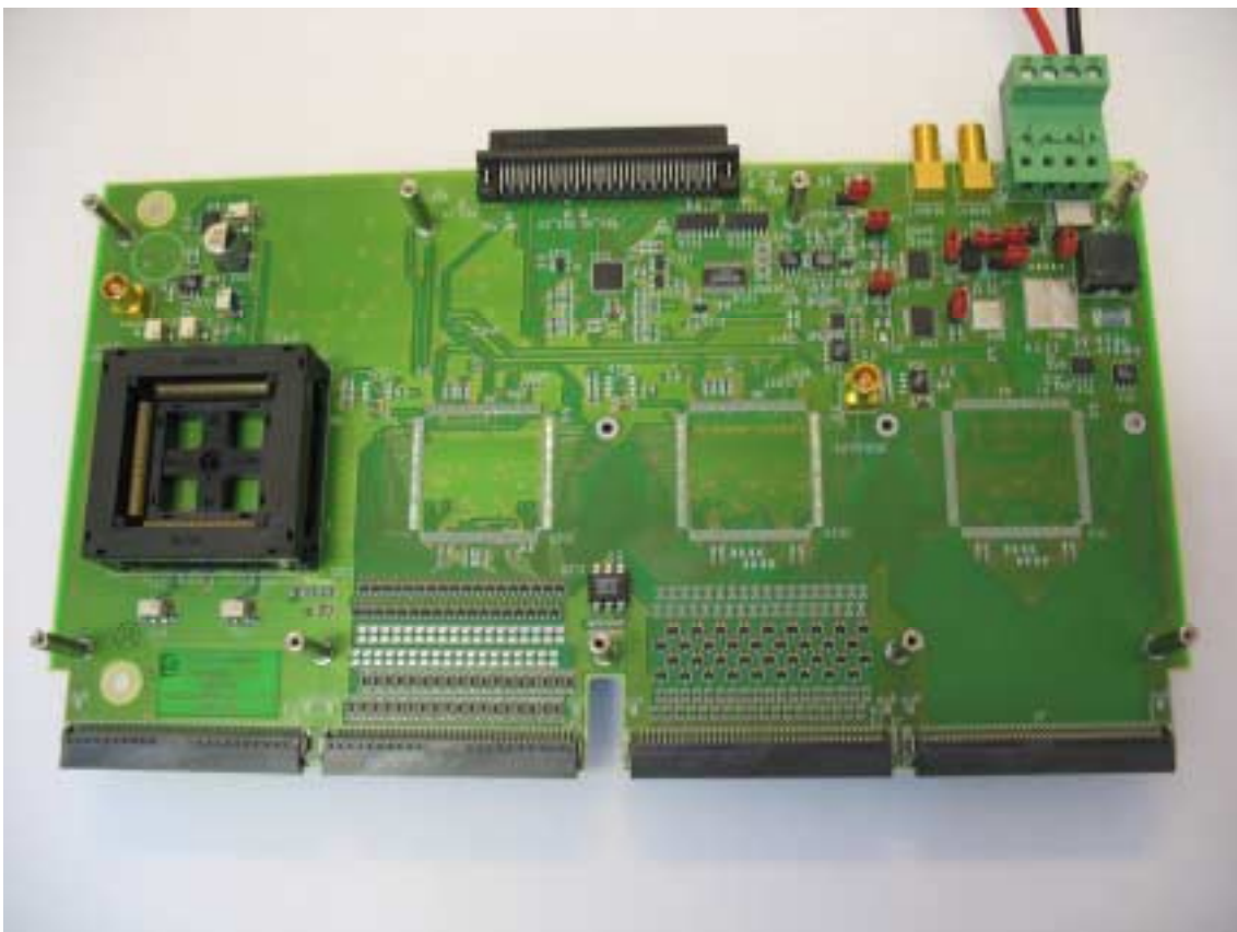
Figure 7 : The After ASIC test board before the ASICs have been progressively cabled. The socket (at left) allows the successive test of a lot of ASIC.
