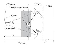
FIG. 1. Experimental setup. The region in the gas volume in which the 10.15 MeV  $^{10}$ Be resonance is formed is indicated (shaded zone). The resonance subsequently decays into  $^{6}$ He +  $^{4}$ He which are detected in coincidence in the LAMP array.
