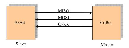
The master and the slave use a protocol based on the following frame structure
