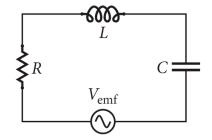
Hints: The voltage across the inductor *leads* the voltage across the resistor by 90°, and the voltage across the capacitor *trails* the voltage across the resistor by 90°. Impedances of the inductor and capacitor are  $\omega L$  and  $1/\omega C$ , respectively, where  $\omega = 2\pi f$ . Note:  $A_{\text{max}} = \sqrt{2}A_{\text{rms}}$ .
