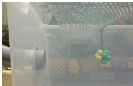
Figure 2. The "target" nucleus attached to a nail hanging from gutter guard that spans the plastic box, beam tube on left.
