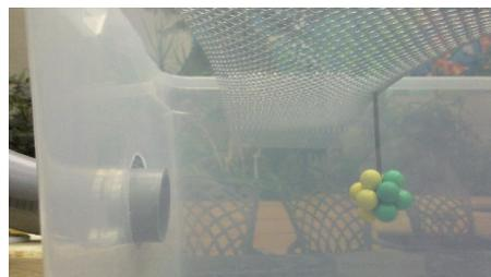
Figure 2. The "target" nucleus attached to a nail hanging from gutter guard that spans the plastic box, beam tube on left.
