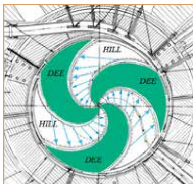
Top-down blueprint of cyclotron interior
