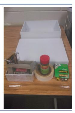
Remove the lid from the box. Pour some iron filings into the box and shake or tap it to make them settle. Put the plastic barrier in the box over the filings (protects visitors). Make sure there's a clear space about twice the size of the box often, the easiest way to set up an experiment is to place the box next to the lid while you're working.
